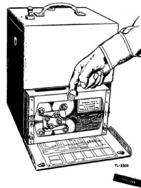
Figure 36. Frequency Meter BC-221-(2), removal of battery tray from frequency meter using finger ring at top.
